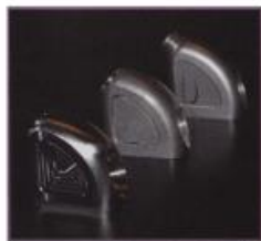
Figure 1: Lean centrifugal processing: this medical device is manufactured from stainless steel. The image on the left shows edge and surface condition as machined edge and surface condition; the middle image shows surfaces after high-speed centrifugal processing, with tool and machining marks fully blended in, and edge and surface requirements met in a mechanical finishing cycle of less than 10 minutes. The one on the right shows the part in its fully configured condition. The lean centrifugal process substantially reduced WIP time and eliminated variables to edge and surface finish. The lean finishing process brought a part-to-part, feature-to-feature, and lot-to-lot uniformity and consistency unattainable with prior methods, and it dropped non-conforming part rates down close to zero.
